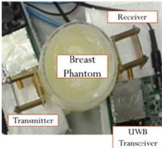
Fig. 4: Experimental set-up
