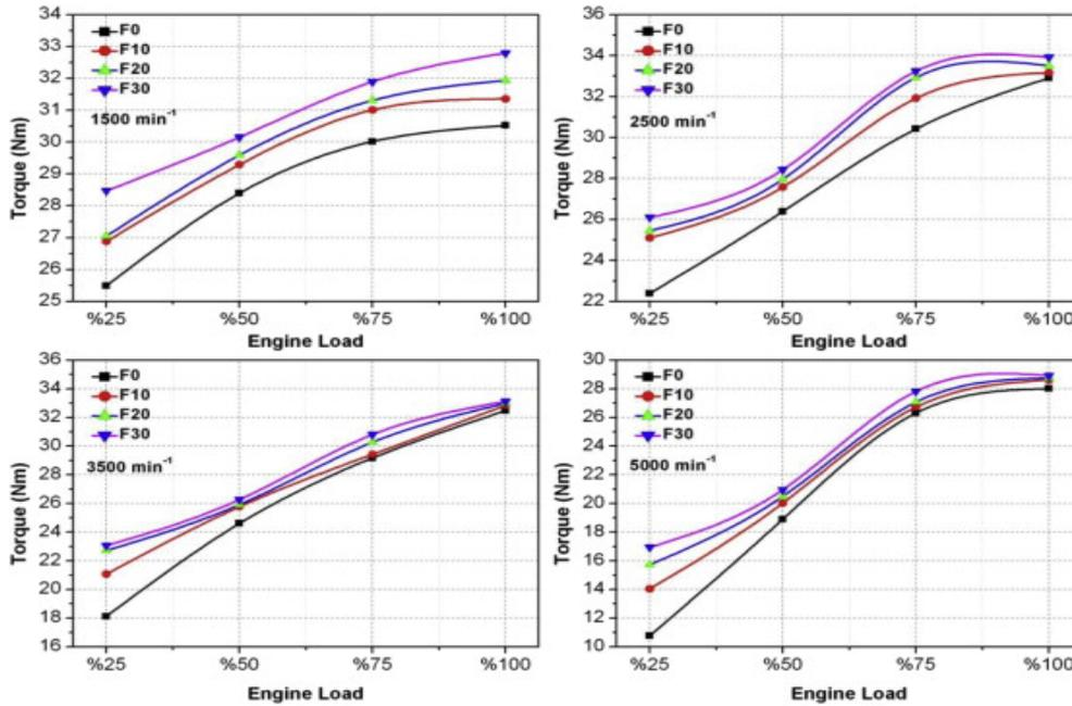
**Fig. 1:** The difference of engine torques with versus engine load at four different engine speeds (Calam et al., 2014)
