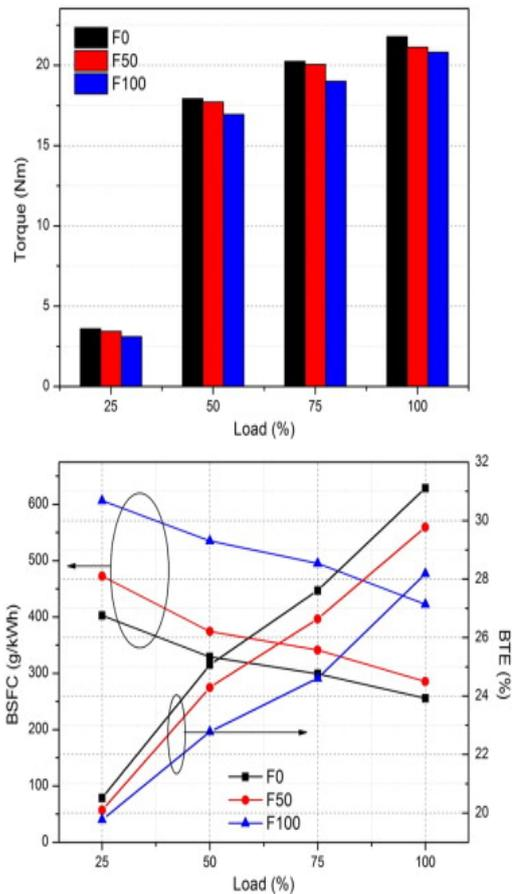
Fig. 2: Torque, brake thermal efficiency and brake specific fuel consumption differences between fusel oil ( F0, F50 and F100) and four different engine load at 2500 rpm engine speed(Solmaz, 2015).
