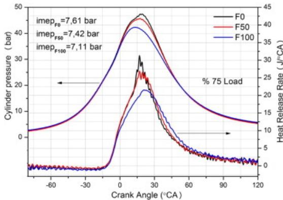
Fig. 4: Impacts of fusel oil on in-cylinder pressure and heat release rate at 100% engine load and 2200 rpm engine speed (Solmaz, 2015)
