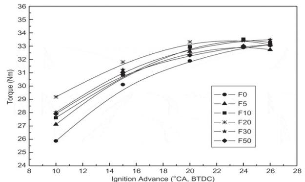
**Fig. 2:** Difference of engine torque with ignition timing (Calam et al., 2013)
