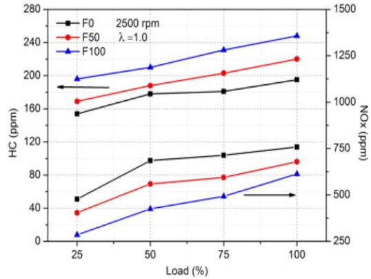
Fig. 5: Impacts of fusel oil on NOx and HC emissions at 2500 rpm engine speed and four different engine load(Solmaz, 2015)
