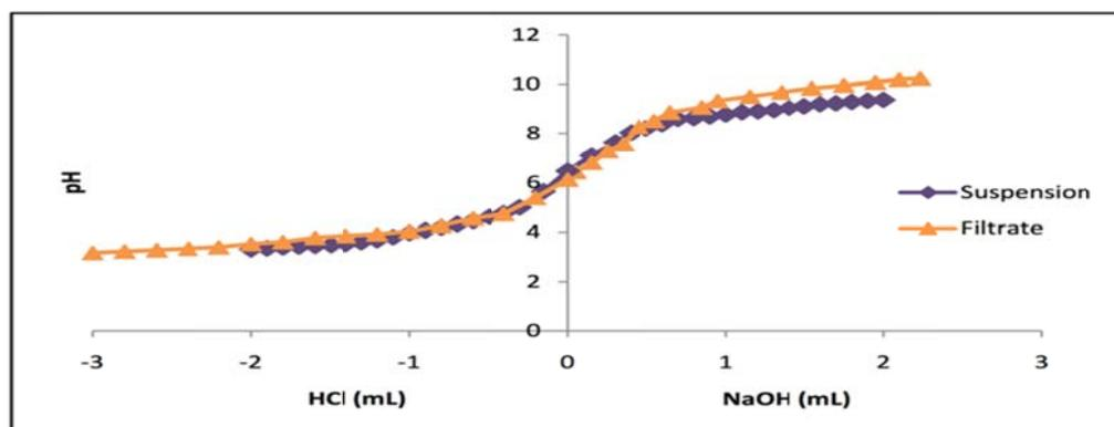
Fig. 5: Titration curve for determination of pH<sub>zpc</sub>
