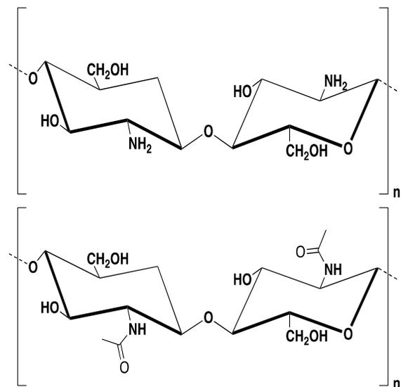
Fig. 1: Structure of chitosan (top) and chitin (bottom)
