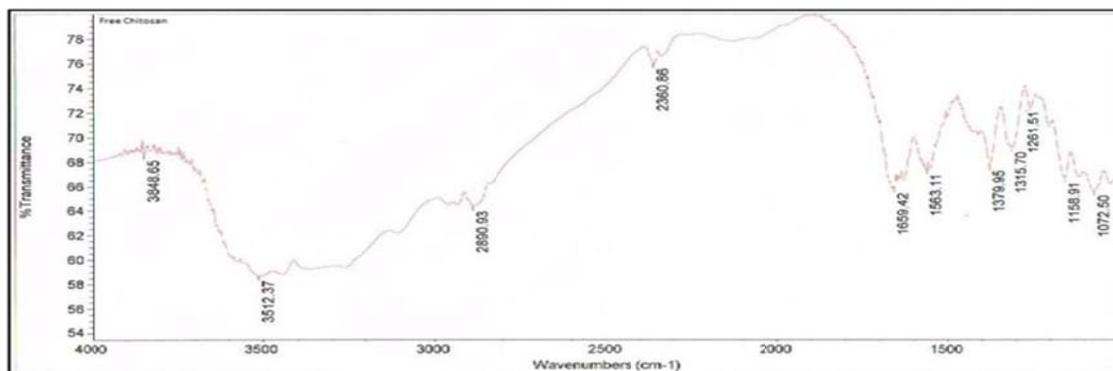
Fig. 4: FTIR Spectrum of "Free" Chitosan
