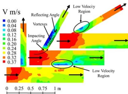
**Fig. 1:** Velocity contours in the plan view for different branching angle and 40% bed width ratio
