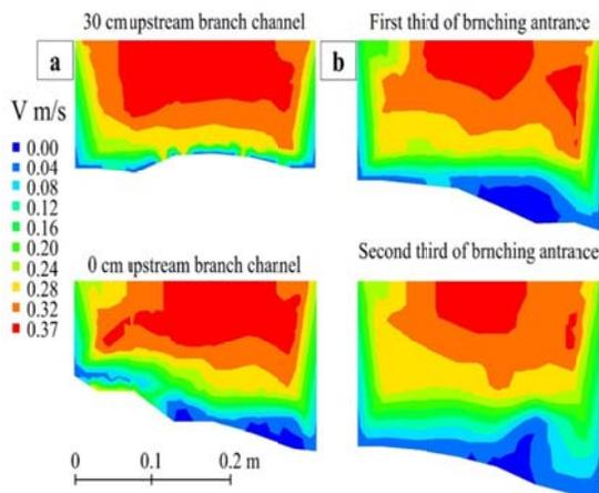
**Fig. 3:** Velocity distribution at cross section of a: upstream main channel, b: along the branch channel entrance, ( $\theta=60^\circ$ ,  $Br=40\%$ , and  $Qt=12.25 \text{ L.s}^{-1}$ )
