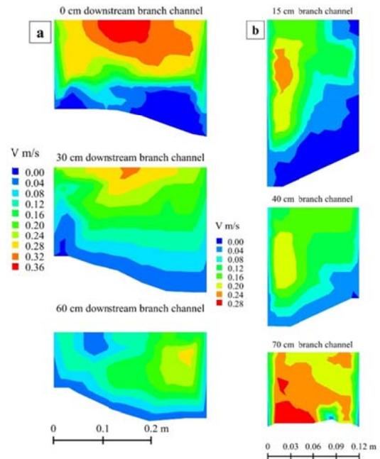
**Fig. 4:** Velocity distribution at cross section of a: downstream main channel, b: branch channel, ( $\theta=60^\circ$ ,  $Br=40\%$ , and  $Qt=12.25 \text{ L.s}^{-1}$ ).
