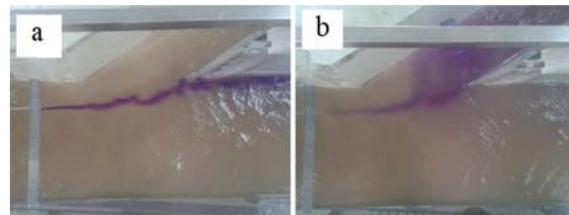
**Fig. 5:** Dye movement to illustrate the upper and lower layers behavior at junction region, at a: 80%, b: 20% from the water depth.
