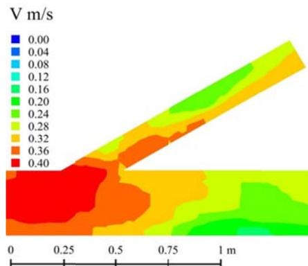
**Fig. 2:** Velocity contour in the plan ( $30^\circ$ , 50% width ratio and  $Q_t=9.75 \text{ L.s}^{-1}$ ).
