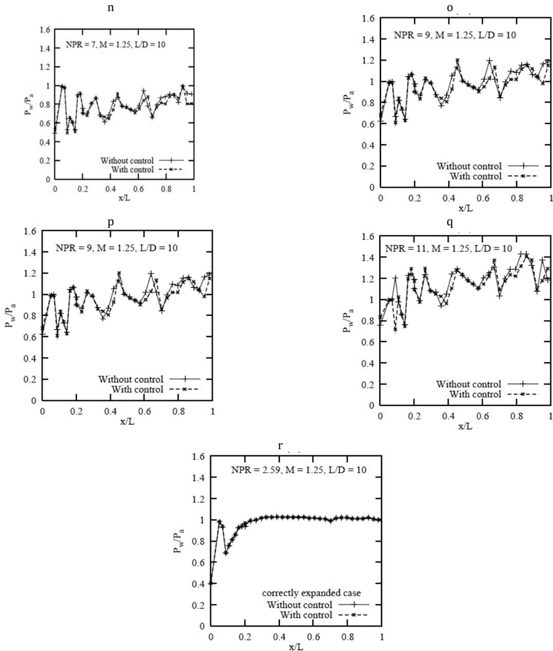
Fig. 7: Percentage change in wall pressure with  $x/L$  ratio (Results for  $L/D = 10$  for NPRs 7, 9, 11, and 2.59)
