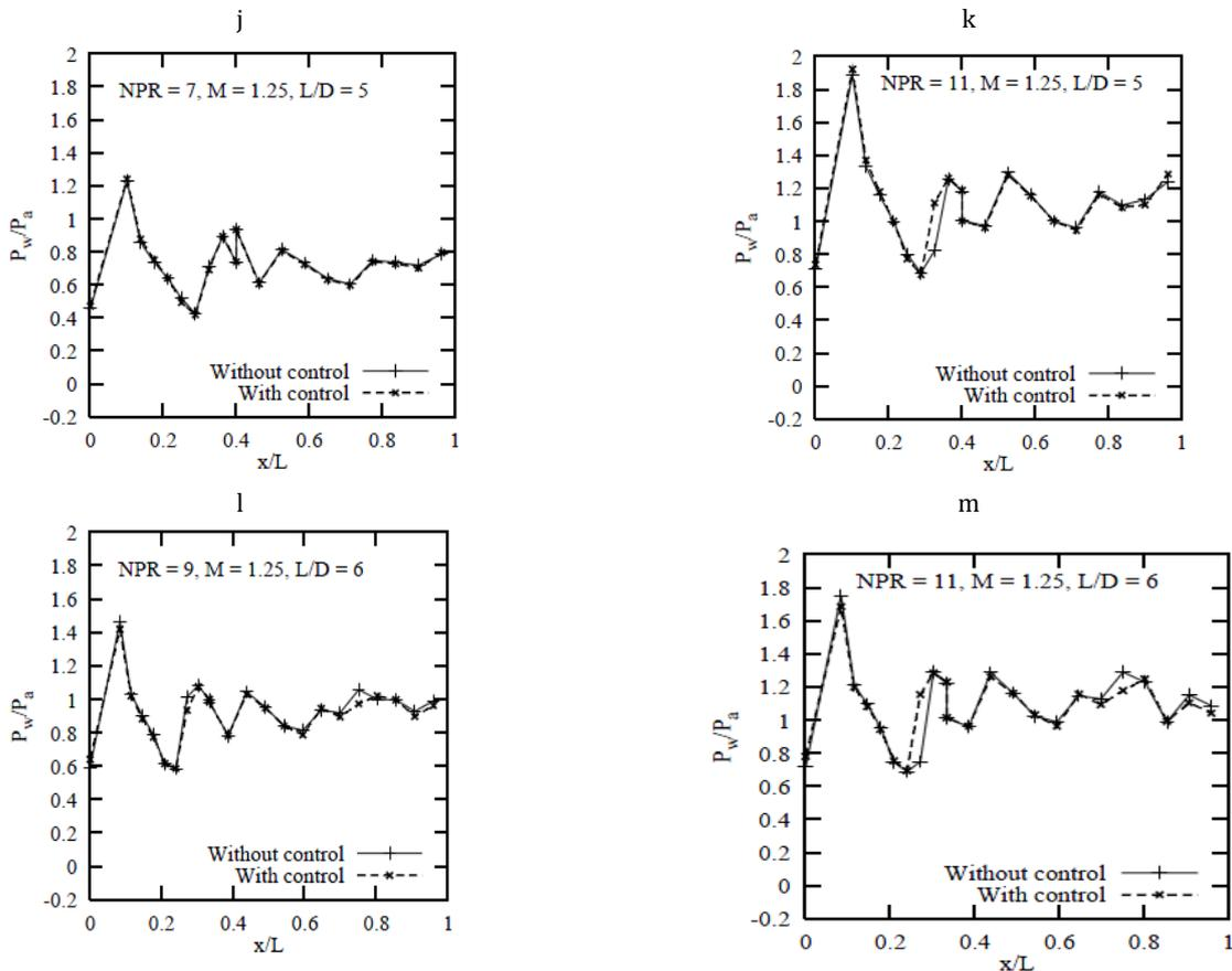
Fig. 6: Percentage change in wall pressure with  $x/L$  ratio (results for  $L/D = 6$  at NPRs 9 and 11)
