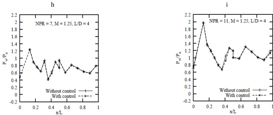
Fig. 5: Percentage change in wall pressure with  $x/L$  ratio (wall pressure results for NPRs 7 and 11 at  $L/D = 4$ )
