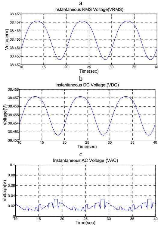
**Fig. 4:** Parameter identification for 2KW PEMFC at 25 °C stack temperature with 15A load: a) instantaneous root mean square b) instantaneous direct current c) instantaneous alternate current
