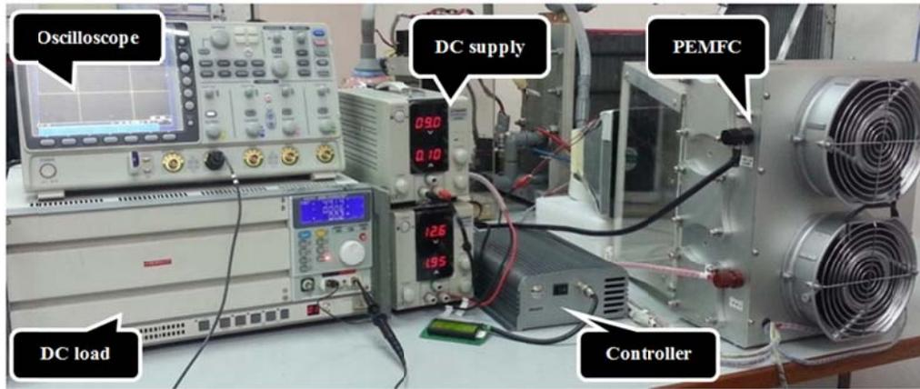
Fig. 1: Experimental setup of H-2000 PEMFC
