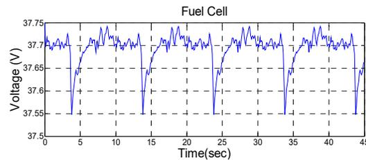
Fig. 2: Time domain information of 2KW PEMFC at 3A load demand with 20°C stack temperature
