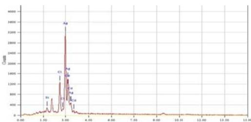
**Fig. 5:** EDX spectrum of the biosynthesized silver nanoparticles
