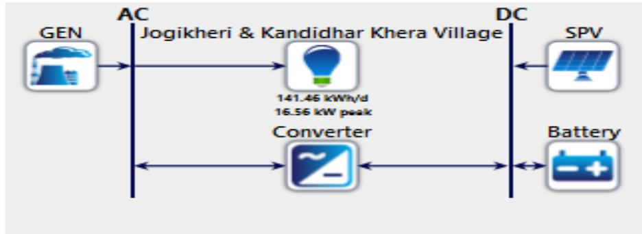
Fig. 2: Proposed hybrid SPV/DG system with battery storage
