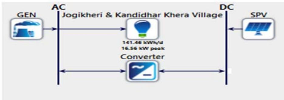
Fig. 3: Proposed hybrid SPV/DG system without battery Storage
