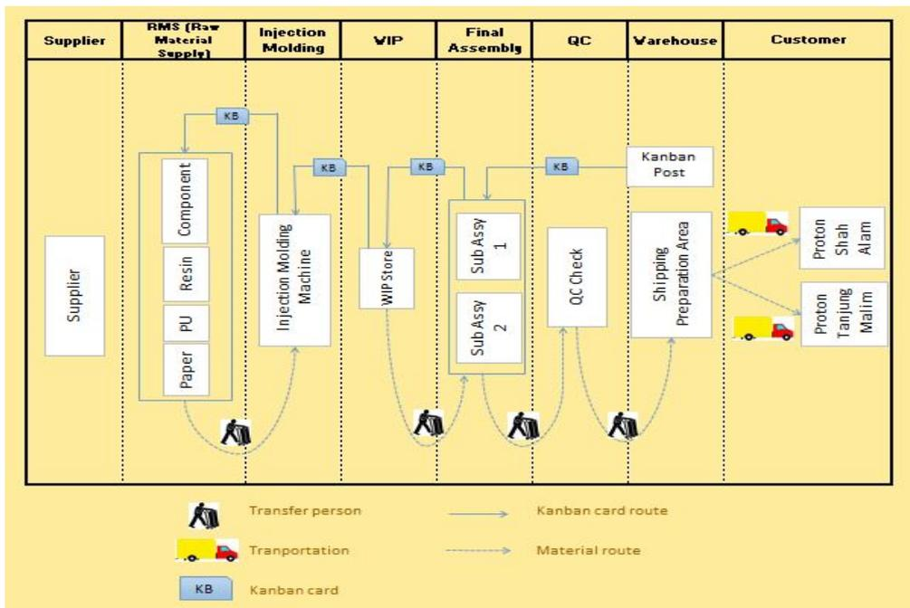
Fig. 1: Material and Information Flow Chart (MIFC) of the research area
