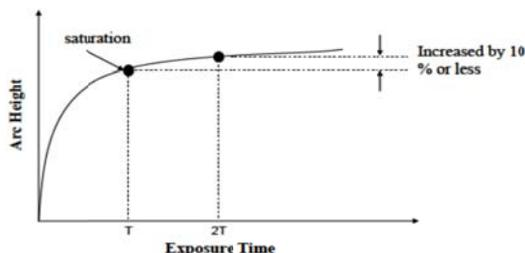
**Fig. 1:** Arc height vs. exposure time scheme(Baiker, 2006).
