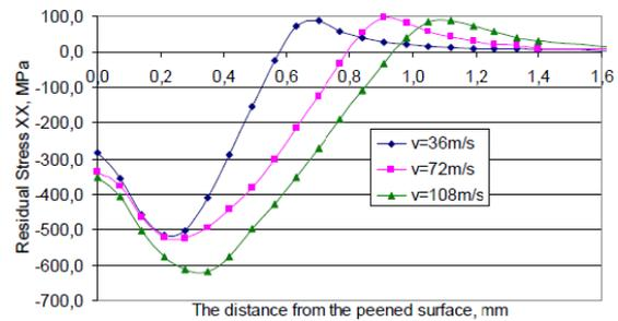
Fig. 2: Residual stress profile for three different shot velocity for a sphere radius  $R = 0.7$  mm.
