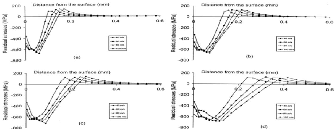
Fig. 3: Residual stress profiles due to shot peening in a thick component, with different shot diameters and at different shot velocities. (a) Shot diameter 0.3mm, (b) Shot diameter 0.5mm, (c) Shot diameter 0.7mm, (d) Shot diameter 1.0mm (Guagliano, 2001).
