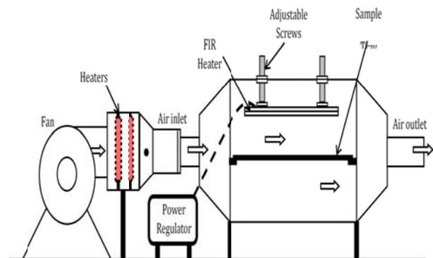
Fig. 1: Schematic view of the infrared drying equipment.
