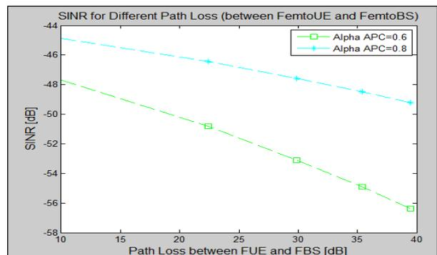
Fig. 6: Graph SINR versus path loss between FUE to FBS by using APC equation
