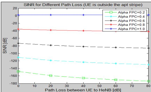
Fig. 4: Graph SINR versus path loss between FUE to FBS by using FPC equation
