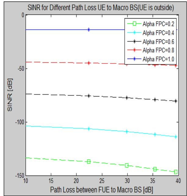
Fig. 5: Graph SINR versus path loss between FUE to MBS by using FPC equation
