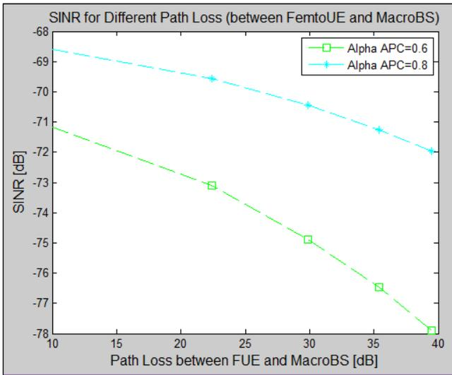
Fig. 7: Graph SINR and path loss between FUE to MBS by using APC equation
