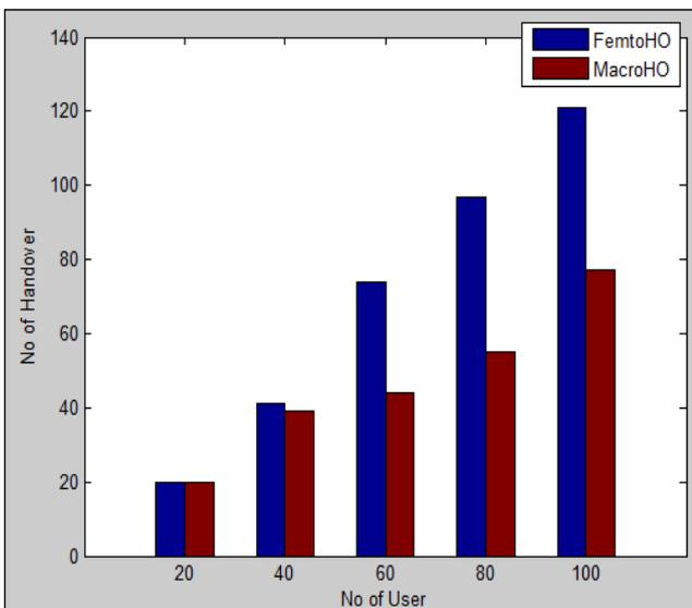
Fig. 11: Number of handovers versus number of users with speed of 20km/h
