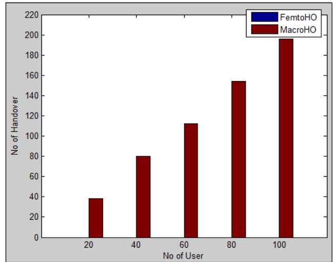
Fig. 12: Number of handovers versus number of users with speed of 100km/h
