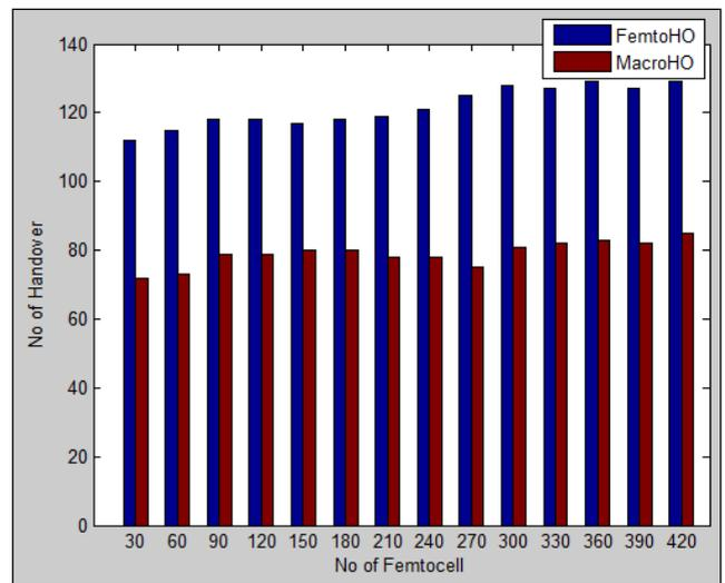
Fig. 13: Number of handovers versus number of deployed femtocells
