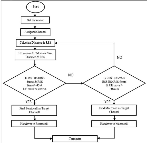
Fig. 3: The workflow of handover scheme
