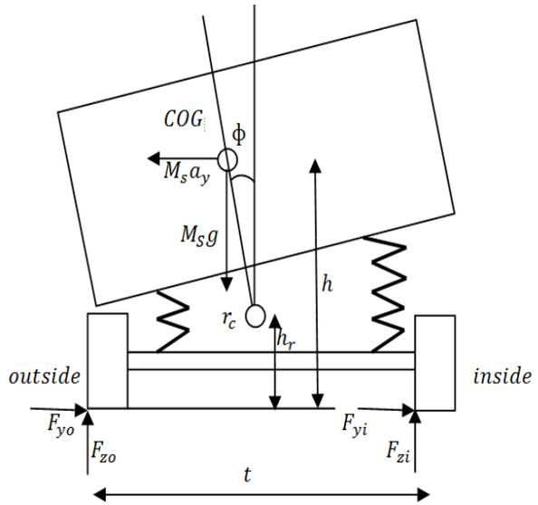
**Fig. 3:** Rollover Free Body Diagram
