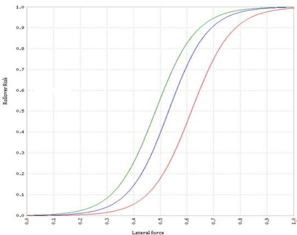
Fig. 9: Rollover risk curve against different lateral force and bank angles
