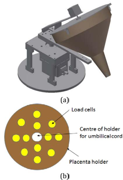
Fig. 5: (a) Proposed structure. (b) Top view of the funnel-like placenta holder from the lid
