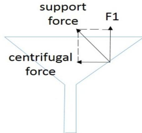
**Fig. 11:** Force Diagram of Secondary Rotation
