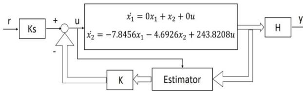
**Fig. 7:** Control Structure without Integral Action
