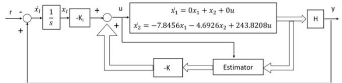
**Fig. 8:** Control Structure with Integral Action
