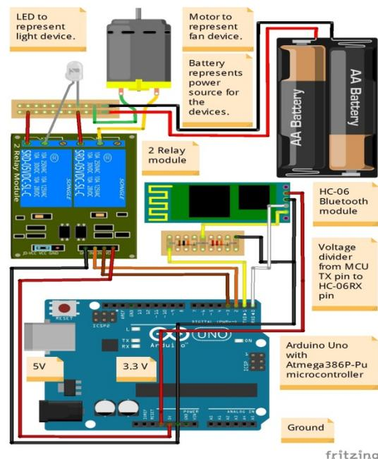
**Fig. 2:** Circuit developed using Fritzing application
