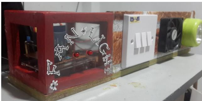
Fig. 6: The completed prototype, with switch, fan and light
