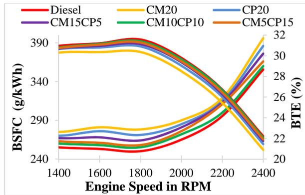
Fig. 3: BSFC and BTE with engine speed variation
