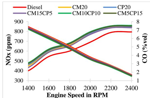
Fig. 4: NO<sub>x</sub> and CO emission with engine speed
