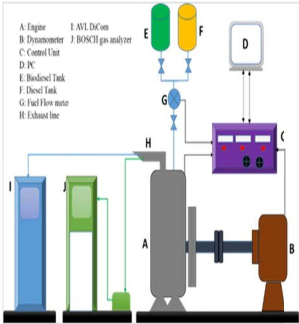
Fig. 1: Engine test bed setup
