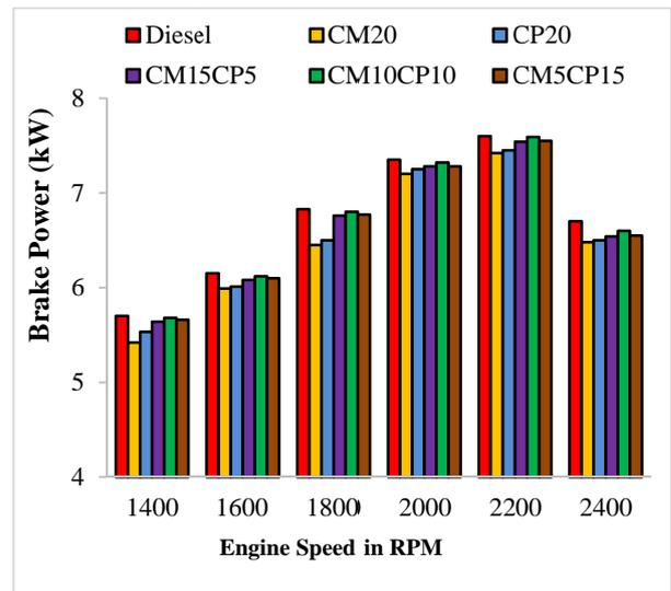
Fig. 2: Brake power with engine speed variation
