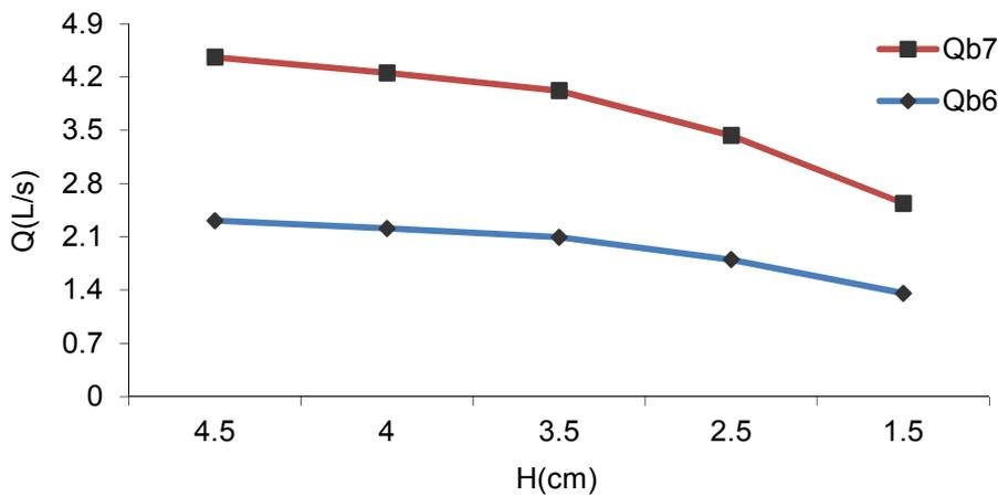
**Fig.4:** Variations the depth flow and discharge against position of blade anti-vortex
