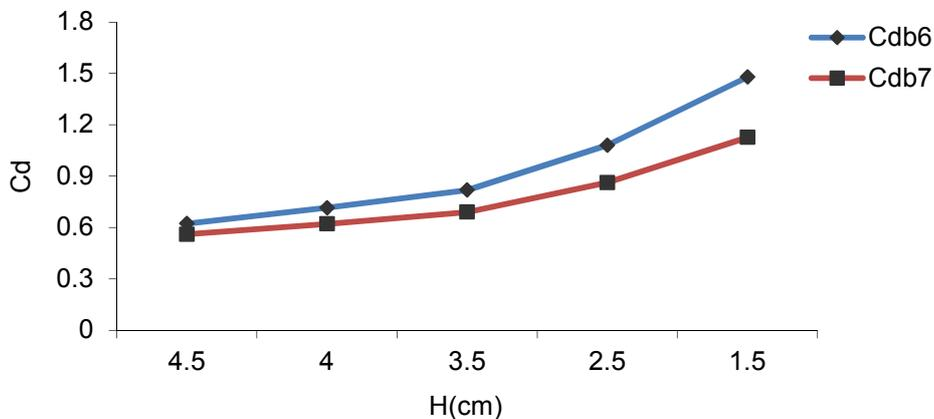
**Fig.5:** Variations the depth flow and discharge coefficient against position of blade anti-vortex
