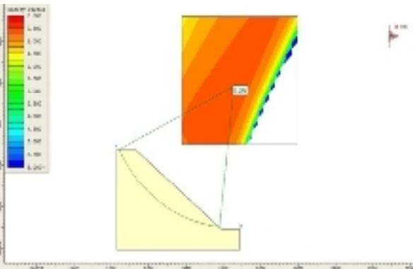
**Fig. 11:** Cut the circle in the debris left by the reservoir with horizontal acceleration 0.5g. (Slope of 40 degrees).
