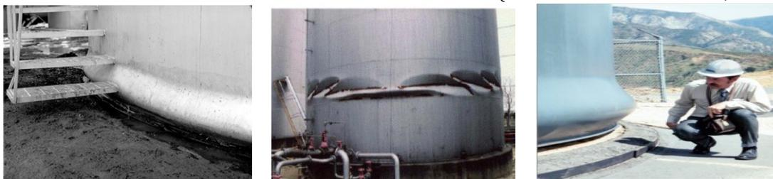
Fig. 3: Types of tank shell buckling
