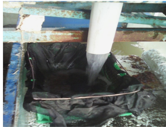
Fig. 3: Discharge output tube and diversion sediment and collecting sediment
