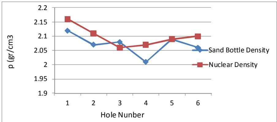
Fig. 1: The comparison of substratum density - test place: part 1 of Kangan bypass
