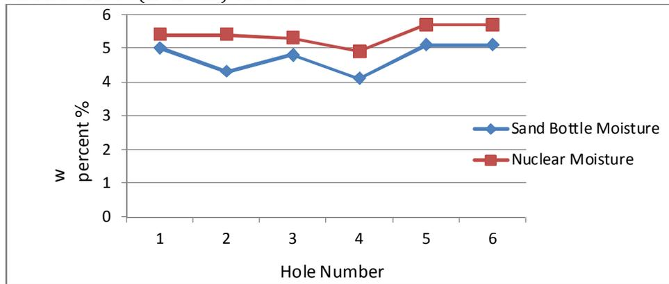
Fig. 8: The comparison of basis moisture – test place: Phase 12- EPC2
