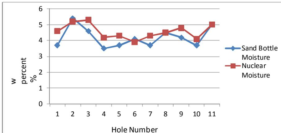
Fig.6: The comparison of basis moisture - test place: part 1 of Kangan by pass
