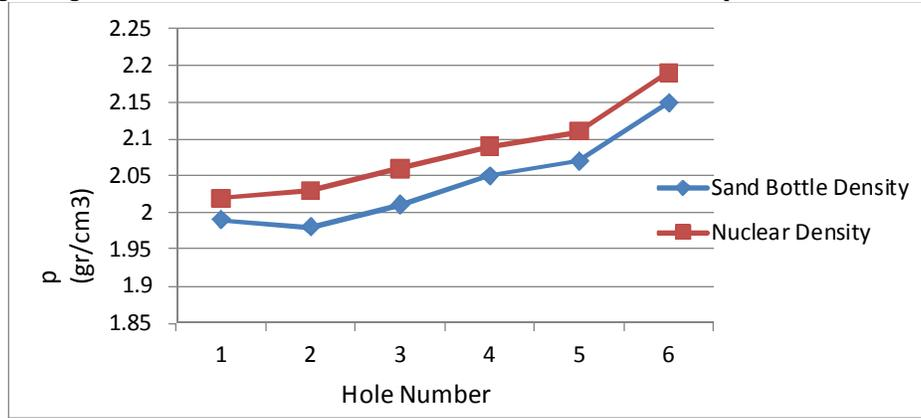
Fig. 7: The comparison of basis density – test place: Phase 12- EPC2
