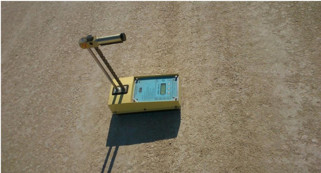
Measurement of density determination and moisture rate by using ASTM1556 and ASTM2216 methods:
