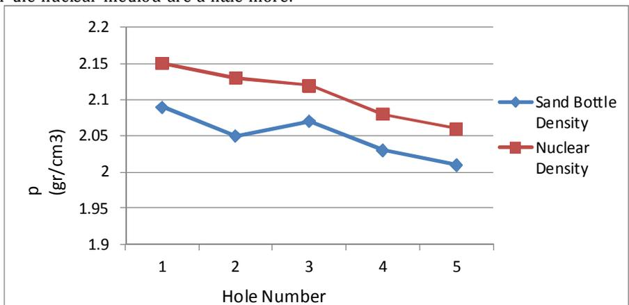
Fig. 3: The comparison of substratum density - test place: Phase 12- EPC2
