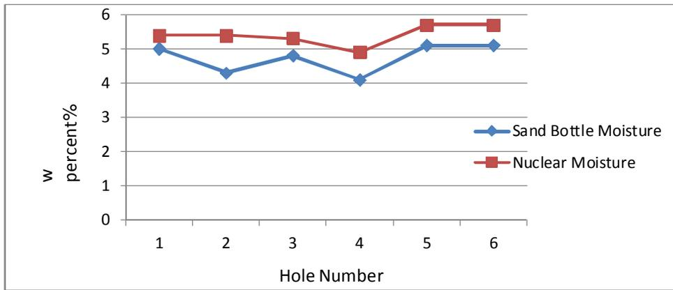
Fig. 4: The comparison of substratum moisture – test place: Phase 12- EPC2
