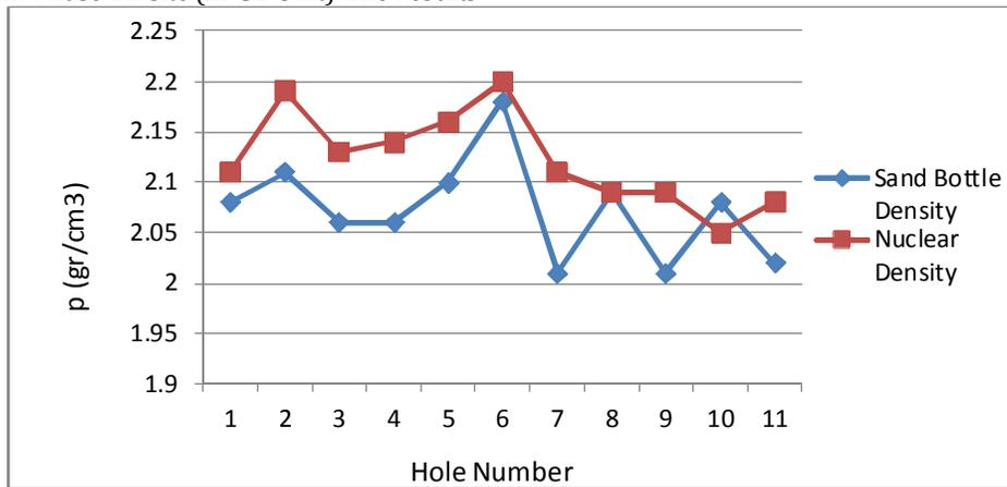
Fig. 5: The comparison of basis density - test place: part 1 of Kangan bypass
