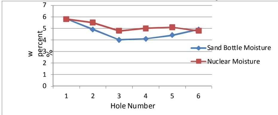
Fig. 2: The comparison of substratum materials moisture - test place: part 1 of Kangan bypass
