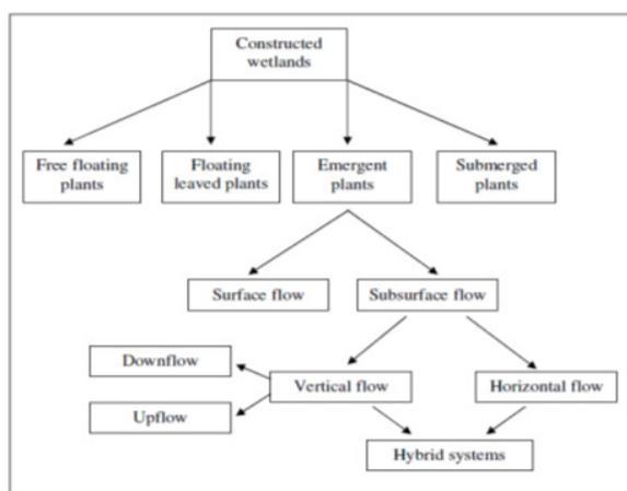
Fig. 1: Classification of constructed wetlands for wastewater treatment (Vymazal, 2001)
