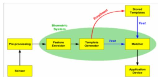
Fig. 1: block diagram of a biometric system
