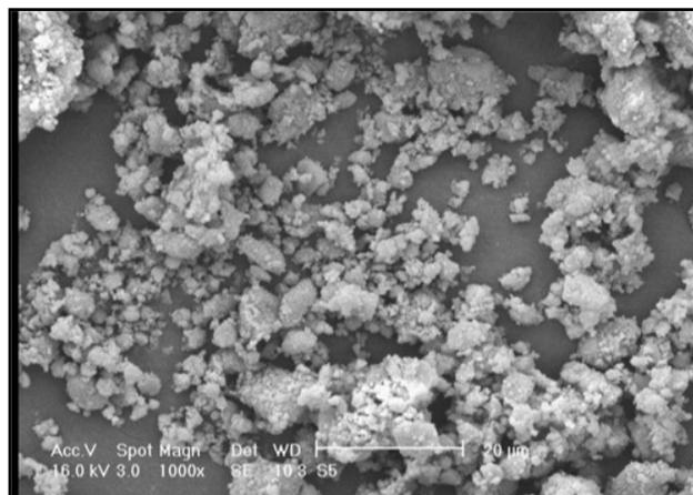
**Fig. 1:** The micro image of the spent catalyst bioleached by acidithiobacillus thiooxidans, taken by a scanning electron microscope (1000 times magnified)
