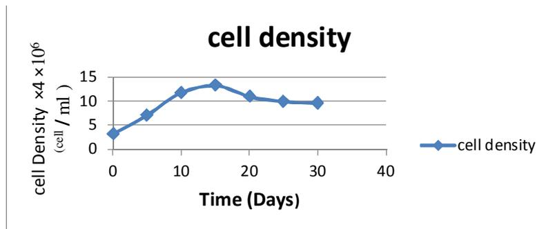
Fig. 4: changes in bacterial population during bacteria-mediated bioleaching of spent catalyst under optimal conditions
