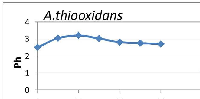
Fig. 2: pH changes during bacteria-mediated bioleaching of spent catalyst under optimal conditions
