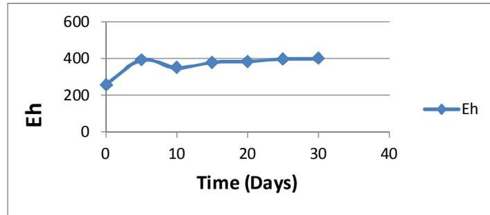
Fig. 3: Eh changes during bacteria-mediated bioleaching of spent catalyst under optimal conditions
