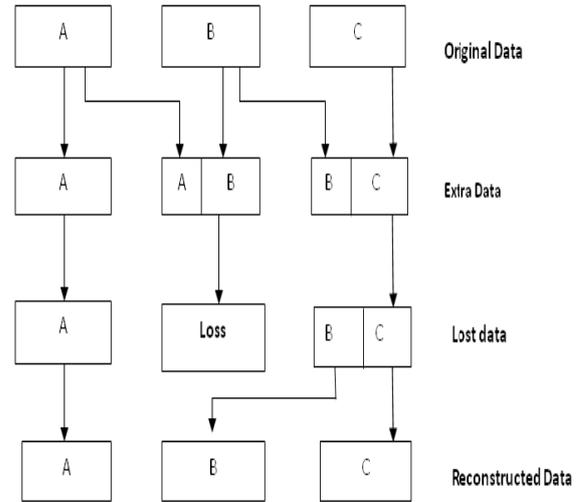
Fig. 5: The procedure of adding extra data and how such data are constructed at the receiver
