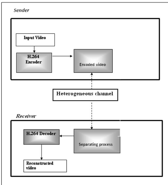
Fig. 1: General system of video transmission over heterogeneous networks
