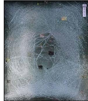
**Fig. 12:** Damages on the laminated glass subjected to 600 gram of explosive
