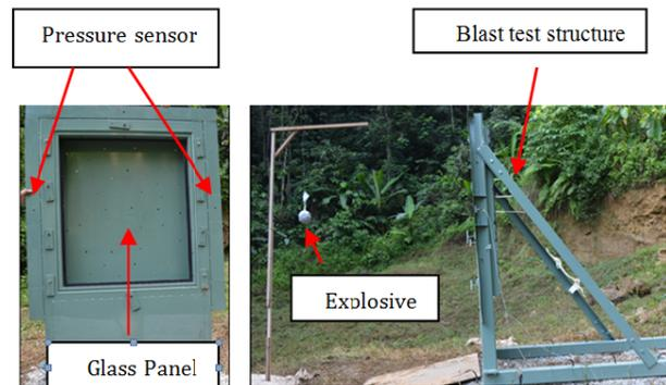
Fig. 3: Field blast test set up
