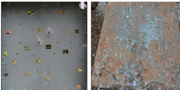
**Fig. 6:** Damaged on the annealed glass panel and also glass fragments due to the blast from 225 gram of explosive.
