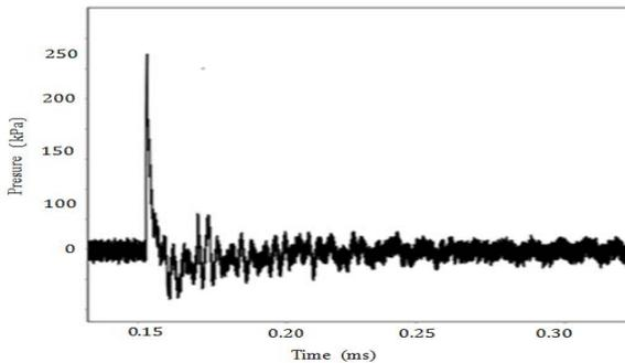
**Fig. 5:** Pressure time history for 7.52 mm thick annealed glass panel subjected to 225 gram of explosive.
