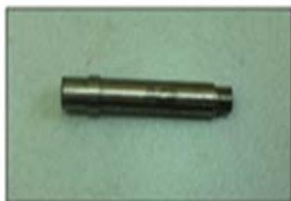
(a) Piezoelectric ICP® Pressure sensor
