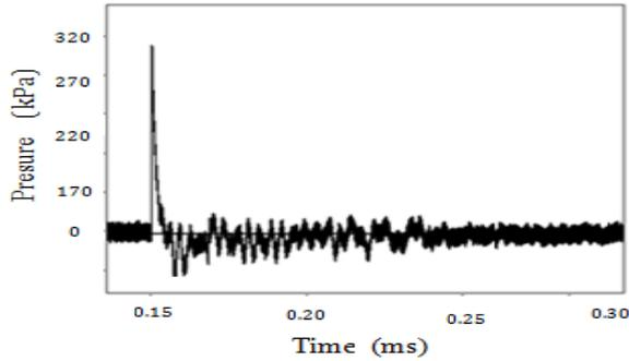
**Fig. 9:** Pressure time history for 7.52 mm thick of laminated glass panel subjected to 300 grams of explosive.
