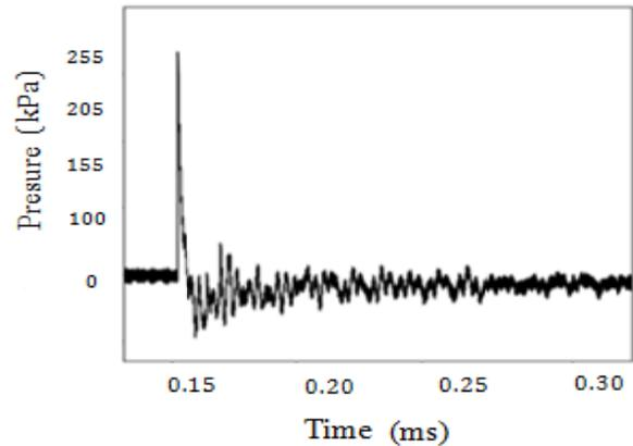
**Fig. 7:** Pressure time history for 7.52 mm thick of laminated glass panel subjected to 225 gram of explosive.
