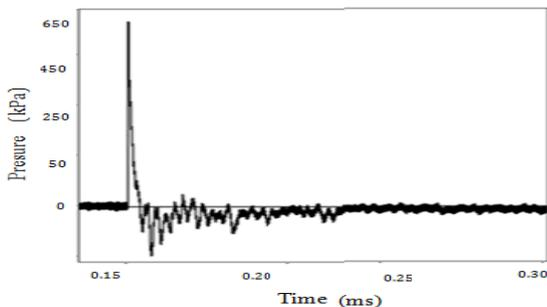
**Fig. 11:** Pressure time history for 7.52 mm thick of laminated glass panel subjected to 600 grams of explosive.
