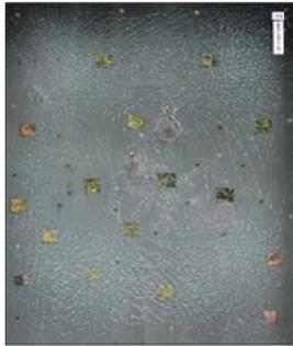
**Fig. 10:** Cracks on the laminated glass panel subjected to 300 gram of explosive
