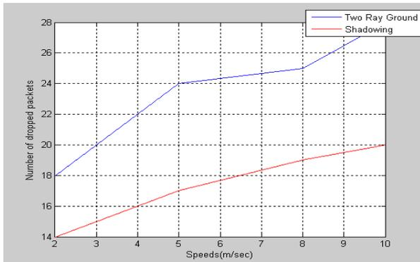
**Fig. 11:** Number of dropped packets for two ray ground model and shadowing
