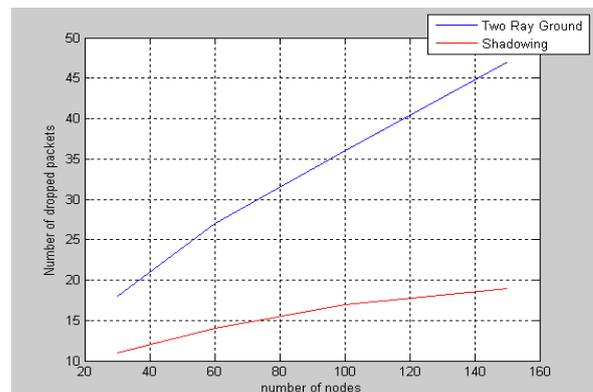
Fig. 7: Numbers of dropped packets for two ray ground model and shadowing
