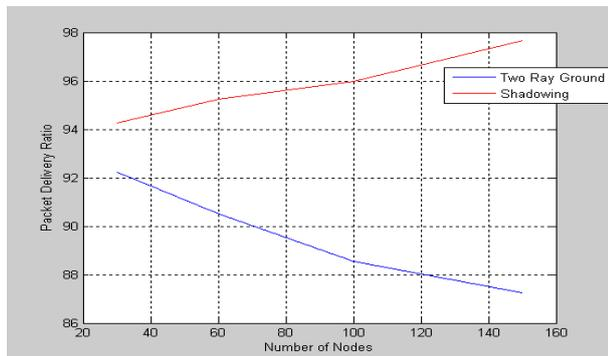
Fig. 5: PDR for the two ray ground model and shadowing
