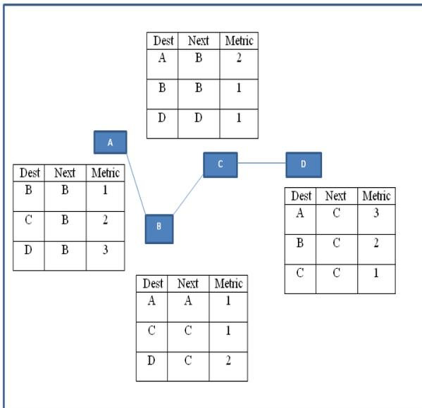
Fig. 2: Distance vector routing
