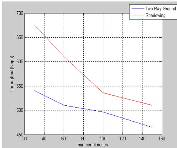
Fig. 4: Throughput for the two ray ground model and shadowing
