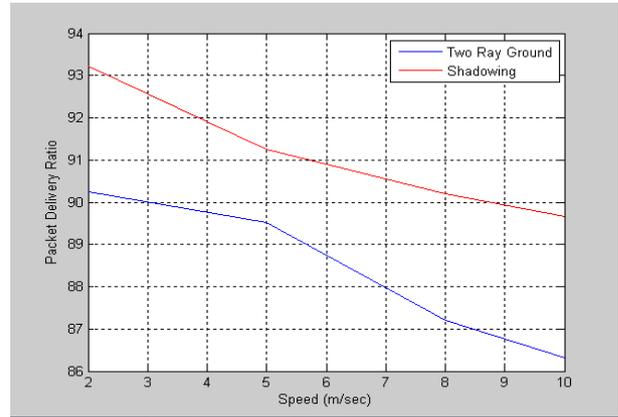
**Fig. 9:** PDR for the two ray ground model and shadowing
