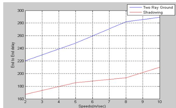
**Fig. 10:** End to end delay for two ray ground model and shadowing
