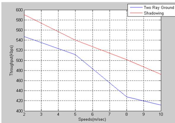
**Fig. 8:** Throughputs for two ray ground model and shadowing
