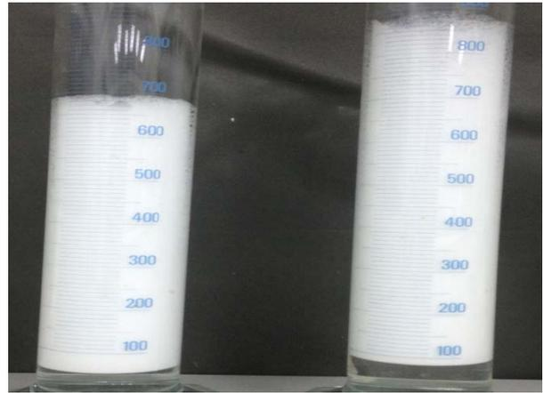
Fig. 6: Foam by N<sub>2</sub> sparging through solution
