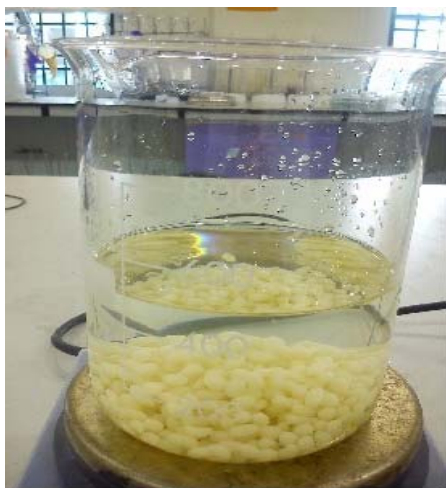
Fig. 1: Immobilized S.cerevisiae in calcium chloride solution
