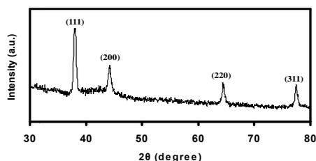
**Fig. 3:** X-ray diffraction diagram of HEC stabilized silver nanoparticles.
