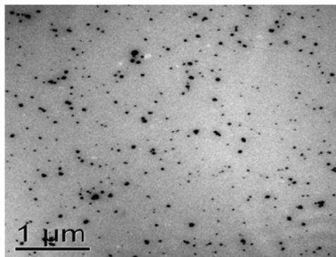
**Fig. 5:** TEM images of HEC synthesized silver nanoparticles.
