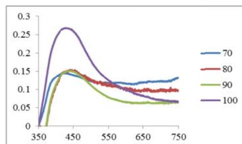
**Fig. 2(c):** The UV-vis absorption spectra of silver nanoparticles synthesized at varying temperature (degree Celsius)
