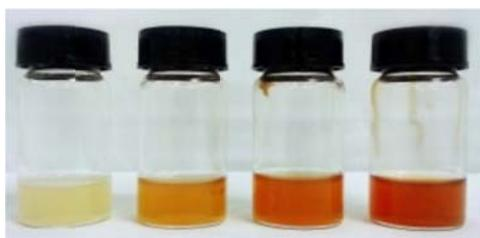
**Fig. 1:** Photograph of Ag-NP suspension at various concentrations of 0.05M AgNO<sub>3</sub>. From left 200, 400, 600 and 800  $\mu$ l
