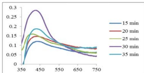
**Fig. 2(d):** The UV-vis absorption spectra of silver nanoparticles synthesized at different reaction time (minutes)
