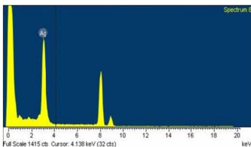
**Fig. 4:** EDS spectrum of silver nanoparticles
