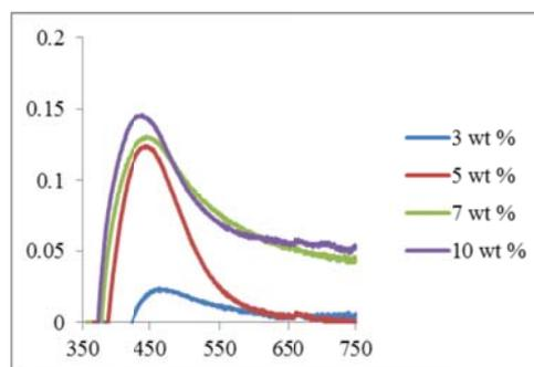
**Fig. 2(b):** The UV-vis absorption spectra of silver nanoparticles synthesized at varying wt. % of HEC.
