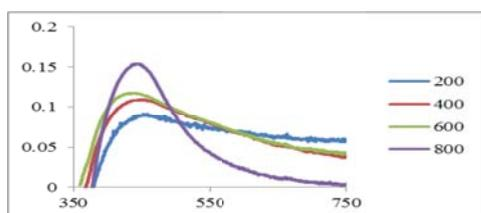
**Fig. 2(a):** The UV-vis absorption spectra of silver nanoparticles synthesized at varying volume ( $\mu$ l) of AgNO<sub>3</sub> (0.05 M)
