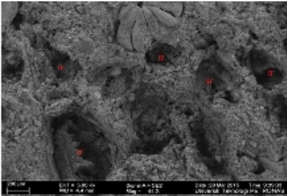
**Fig. 18:** Intrafossil (IF) pores
