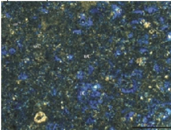
**Fig. 14:** Mudstone texture, mainly micrite (µC) with intercrystalline pore in blue
