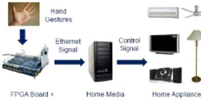
**Fig. 9:** Hardware setup of the proposed system
