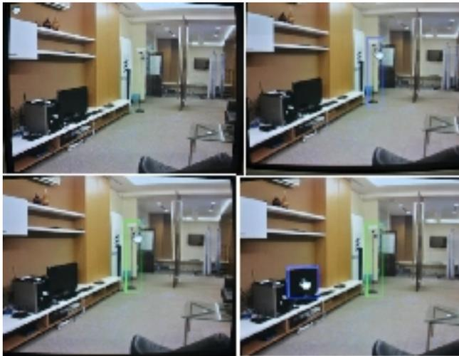
**Fig. 12:** (a) User Interface (b) Selected lamp via cursor (c) Lamp turned on (d) Selecting TV for control
