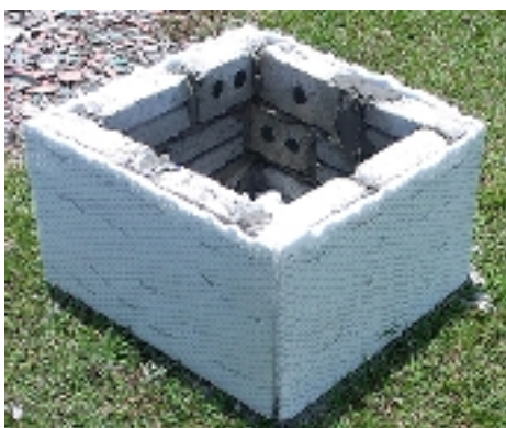
Fig. 3: Sand brick wall that apply polystyrene before plastering
