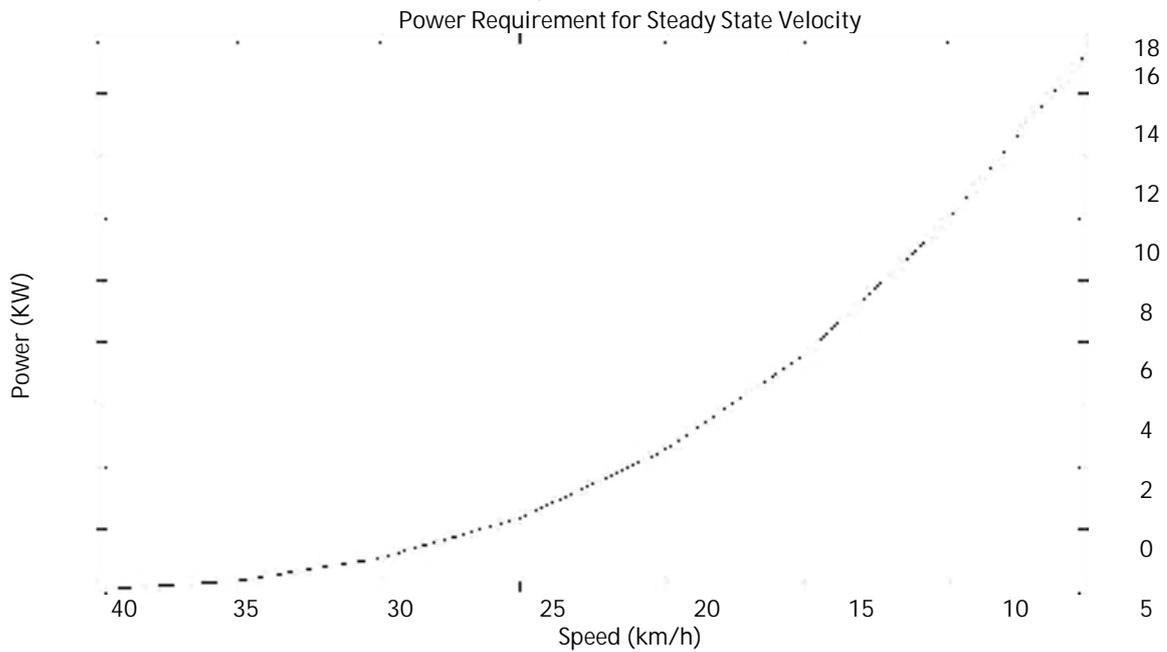
Fig. 3: Boat power requirements for steady state velocity
