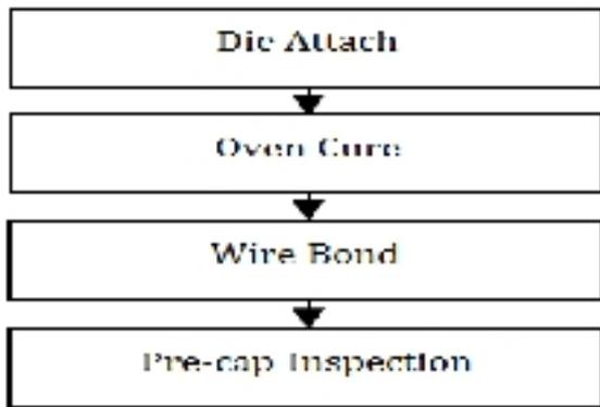
**Fig. 2:** Semiconductor manufacturing process flow
