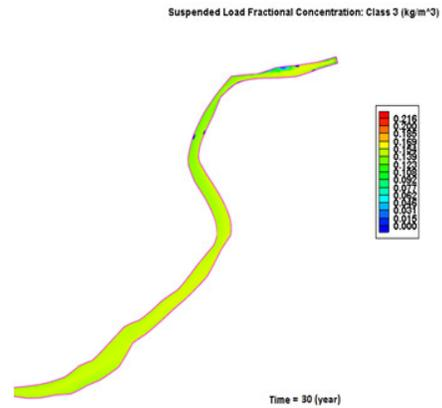
Fig. 7: Suspended load concentration for class 3
