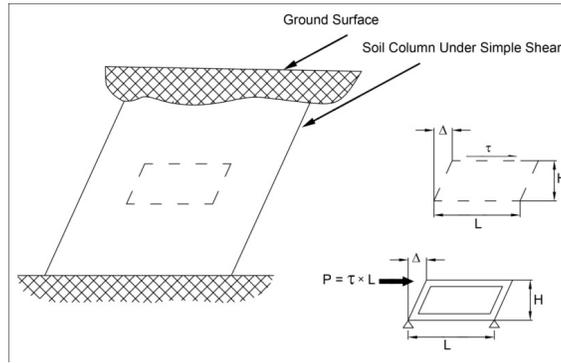
Fig. 5: Soil relative stiffness and a rectangular frame
