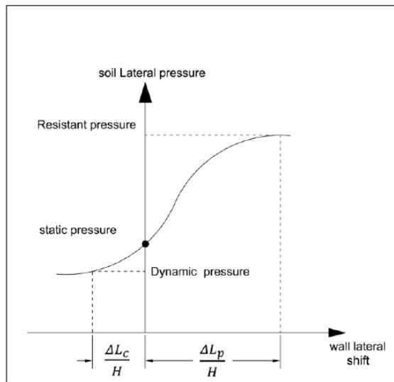
**Fig. 1:** Soil lateral displacement versus structure displacement
